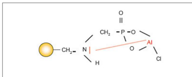
Figure 1: Functional Group Of The AMPA-Resin Lewatit MonoPlus® TP 260 After Loading With Aluminum-Chloride
