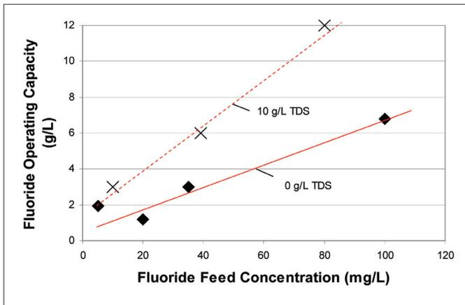
Figure 6: Effect of feed concentration on operating capacity under two different operating conditions: With 10 g/L total dissolved solids (TDS) in the background and with demineralized water background (0 g/L TDS). Specific Velocity (SV) = 10 BV/h, 1.3 moles of  $Al^{3+}$  doped per liter of resin Lewatit MonoPlus® TP 260, feed pH = 3.6; salt mixture for TDS background containing 50% p.w. NaCl and 50%  $Na_2SO_4$ .
