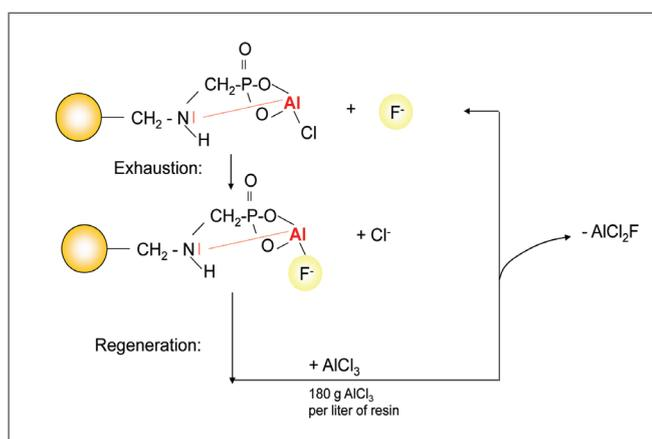
Figure 2: Reaction Scheme Of The Selective Fluoride Removal By Aluminum Doped Lewatit MonoPlus® TP 260
