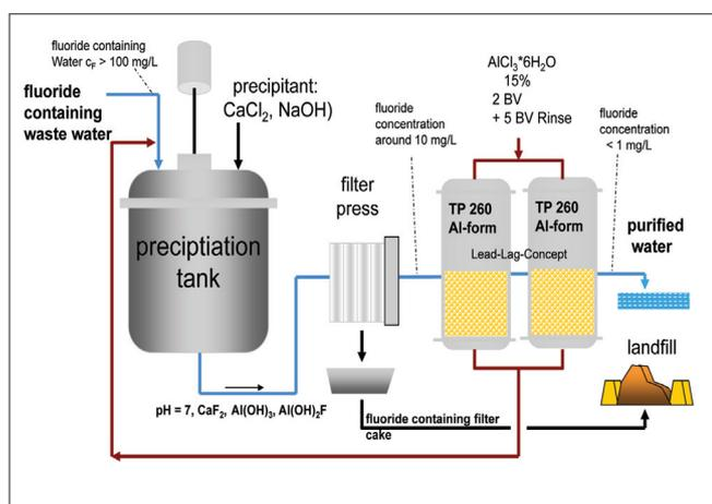
Figure 3: Principle Of Using Fluoride Selective Resin As A Polishing Filter Unit Behind  $\text{CaF}_2$  Precipitation
