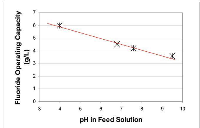
Figure 7: Effect of pH on fluoride operating capacity. SV = 10 BV/h, 1.2 moles of  $Al^{3+}$  doped per liter of resin Lewatit MonoPlus® TP 260, concentration of fluoride in feed = 127 mg/L, demineralized water background
