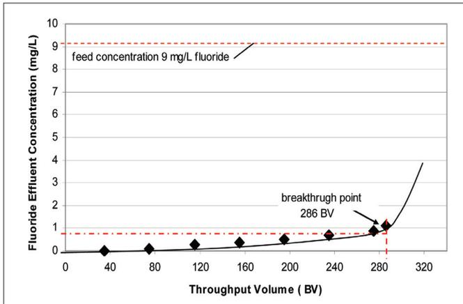
Figure 5: Original Filtration Curve Generated From Data Measured At The Gujarat Reference Plant.
